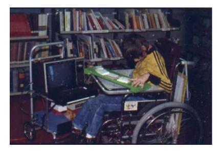
In the above photo is shown a 5 key user The : keys are made from commercial light switches with the actual switching mechanism replaced by micro-switches,
