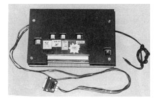
The above photo shows a 5 key keyboard used in the first stages of the project. This keyboard was adapted from an ordinary ASCII keyboard by shielding out most keys. Only the more accessible key, the space bar, was used for time-slot selection -- this was the ZAP key. All the other four keys could be struck at any time independently of the location of the cursor to execute a function as marked.
